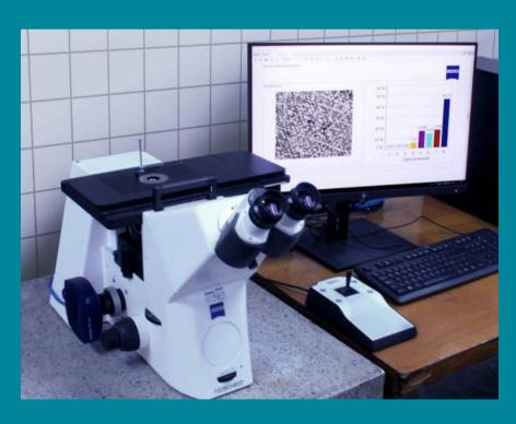
Inverted plate metallographic microscope
